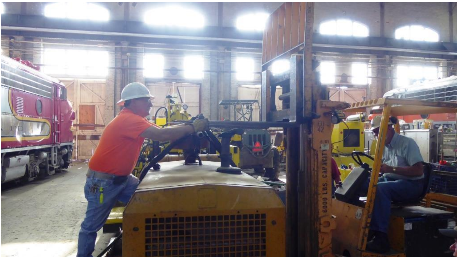
Mike H. gets a strap wrapped around the engine for Alan on the fork-lift to lift
