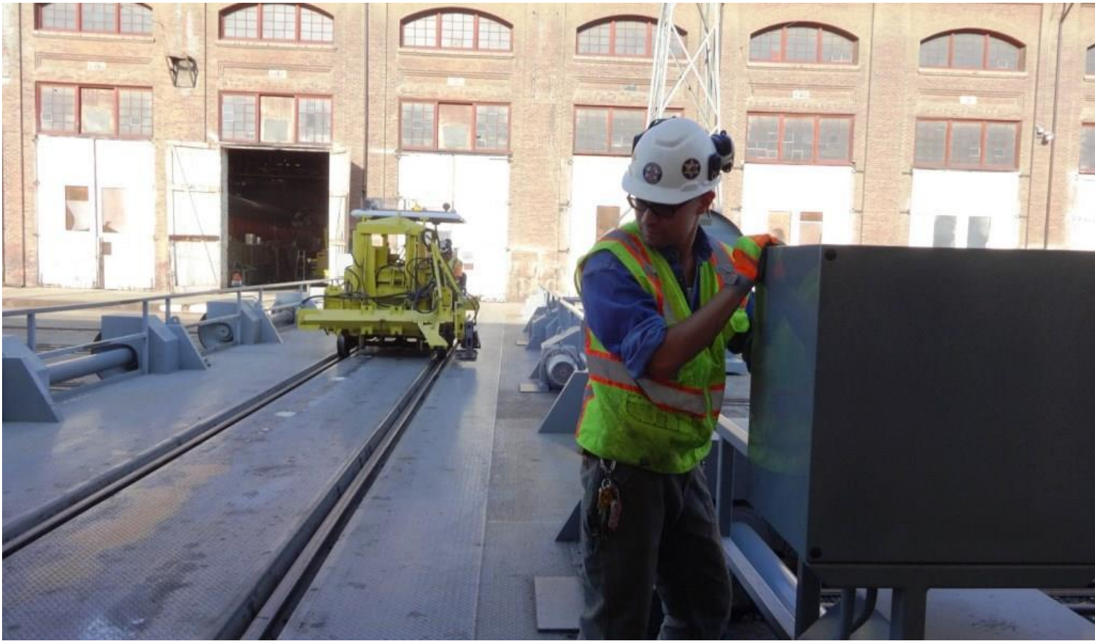
Kyle runs the transfer table as the Jackson 125 tie-exchanger is moved to the transfer table lead track
