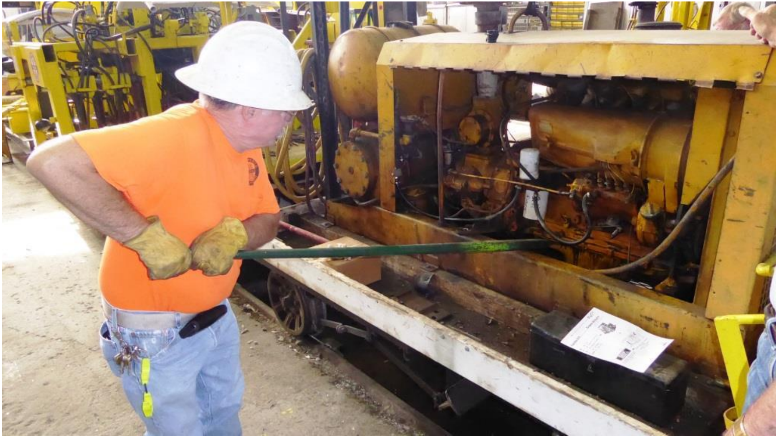
Mike H. uses a lining-bar to lever-up the air-compressor's Deutz air-cooled diesel engine
